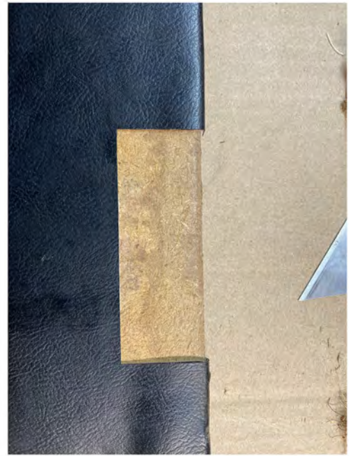
Fig. 8a Cut out this section from the panel completely.
