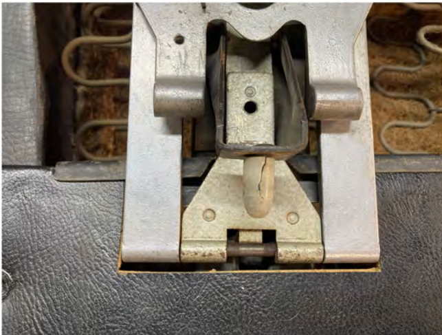
Fig. 8b Install the panel. It should now sit around the hinge.
