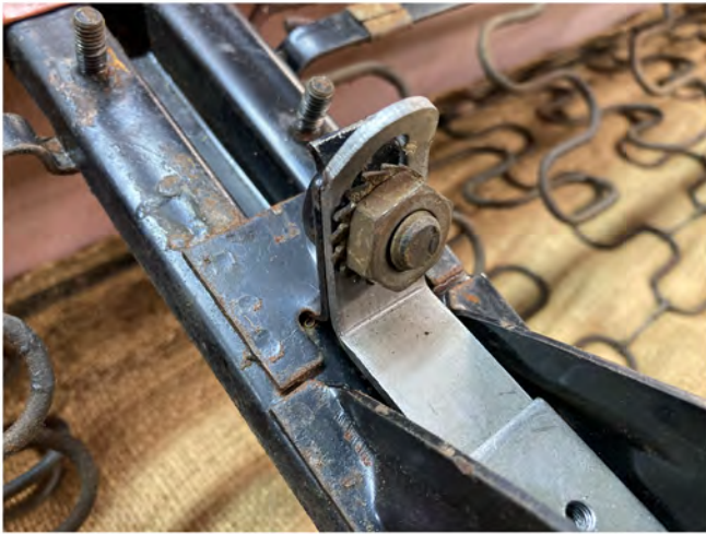
Fig. 1 Attached the hinge to the rear seat.
