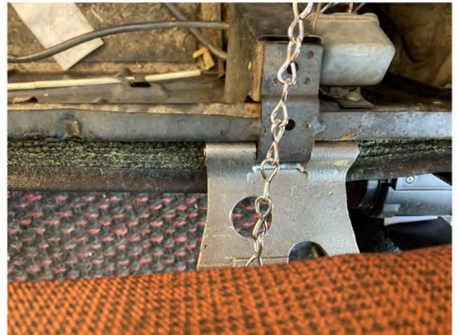
Fig. 9 Install the seat back into the vehicle. Install the hinge pins through the hinge and seat base.
