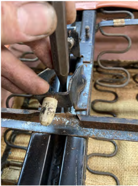
Fig. 5 Peen this flat with a punch or smooth with a file.
