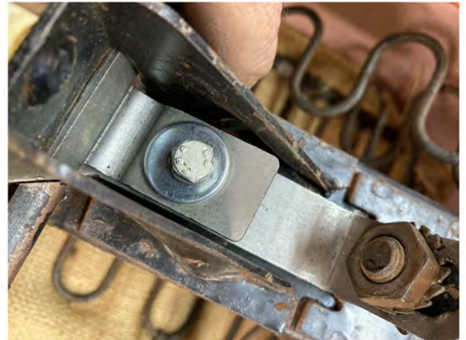
Fig. 6a Secure the bracket to the hinge.
