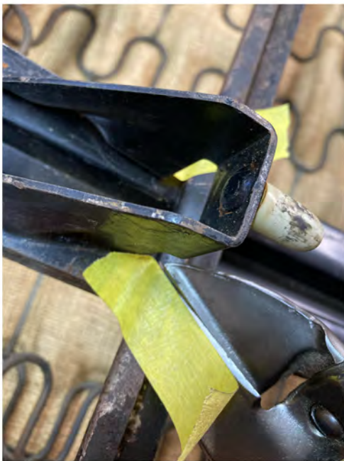
Fig. 3 Cut the U-Channel with tinsnips.
