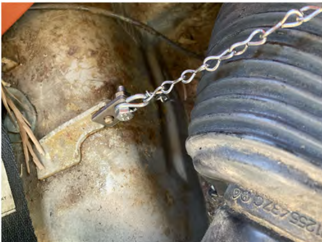
Fig. 10 Install the chain bracket onto the body. Secure with c-clip (not pictured).
