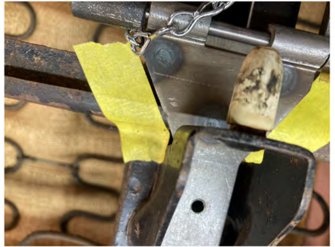
Fig. 2 Mark the U-channel with tape or a marker.
