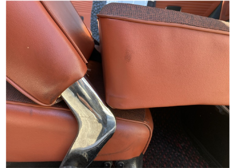
Rest the front of the rear seat on the front seat bottoms.
