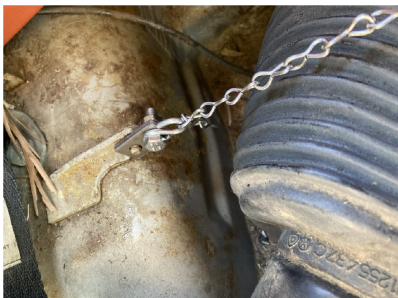
9a Chain bracket on the body, secured with a c-clip (not pictured).
