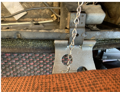
8a Drive the pins through the hinge and seat base.
