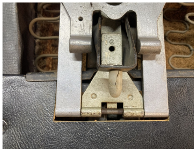
6c The panel now sits around the hinge.
