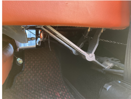
Hinges extended into the camping bed.
