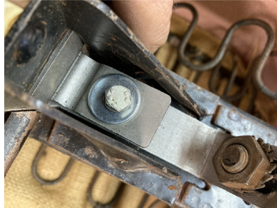
7b Secure the bracket to the hinge.
