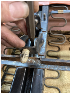
5e Peen flat with a punch or smooth with a file.
