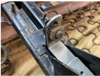
3a Hinge attached to the rear seat.
