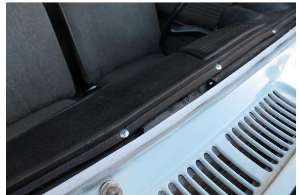
Large-head screws securing the leading edge on an earlier car. Paint the heads black so they blend in with the pad.
