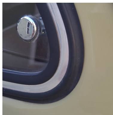
Installed correctly, with the bright frame band showing.
