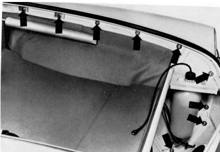
D Step 7: Screws inside the front luggage compartment
