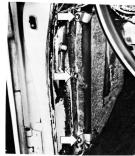
C Step 5: Bolts behind the front side trim panel
