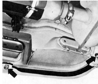
C Step 8: Lower rear fender mounting screws
